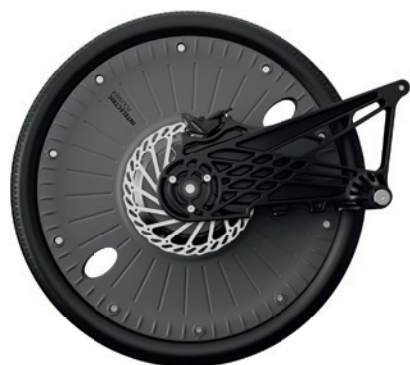
Assembly configuration (rear): icoMR1500.24/iBRS/iSA
